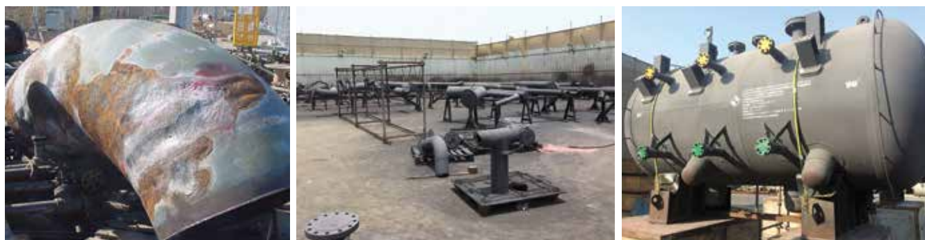
FIGURE 5. Severe corrosion under insulation (CUI) resulted in this instance (above, left) from a zinc-based primer, which is not recommended for closed, wet environments. At temperatures greater than 60°C, the zinc may undergo a galvanic reversal in which it becomes cathodic to carbon steel. The MIO/IMM coating (Heat-Flex® Hi-Temp 1200) is applied direct-to-metal to large pipes, valves (above, center) and tanks (above, right) before shipping to the construction site. The coating is effective in protecting components from corrosion in ambient C5 environments or at high heat under insulation.
